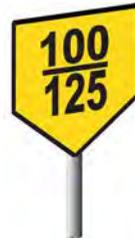
Warning indicators are provided on the approach to certain EPS speed indicators and give a warning of a reduction in the enhanced permissible speed ahead.
