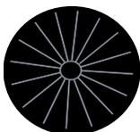
The black indication advises the driver that the associated signal is showing a green aspect or 'all clear'. It also advises the driver that the audible warning has not been acknowledged and, if not acknowledged, the brakes will be applied.
