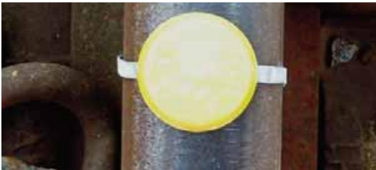
**Detonator secured to rail**
