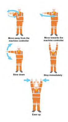
Diagram HB.15.2 Handsignals during daylight
