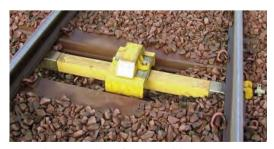
An example of a portable magnet
