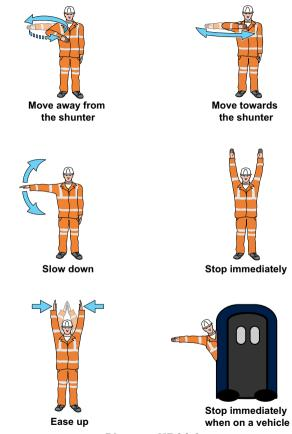
Diagram HB14.1 Hand signals during daylight
