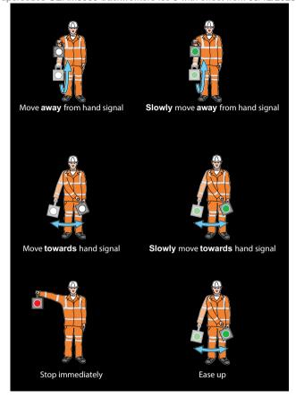
Diagram HB14.2 Hand signals during darkness or poor visibility
