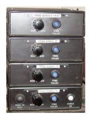
Example of a failure indication unit
