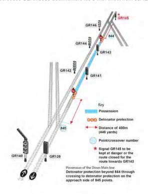
Diagram HB11.2 Standard detonator protection - points involved
