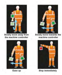
Diagram HB15.3 ERTMS Handsignals during darkness or poor visibility
