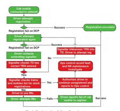
Fig 1. Registration failure flowchart
